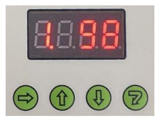
As shown in the figure above, the current display content of the digital tube is 1.98, and there is a red decimal point in the lower right corner of the digital tube of the number 1, which represents the current number as the changeable item of the menu option;
