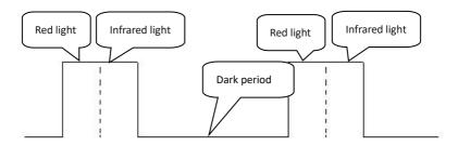
4, red and infrared light continuous light, no dark interval in the middle or dark interval is very small, less than 100us, as shown in the following figure:
