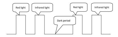
3, red and infrared light continuous light, no dark interval in the middle or dark interval is very small, less than 100us, as shown in the following figure:
